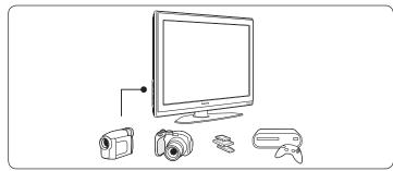
Use the TV side connectors to connect to mobile devices such as a camera or high definition game console. You can also connect a pair of headphones or a USB memory device.
